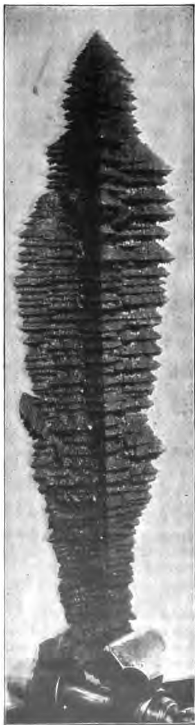
Fig. 5. Steel Crystal, about half natural size. From the collection of Professor Tschernoff. ( The Metallgraphist , II, p. 74.)
